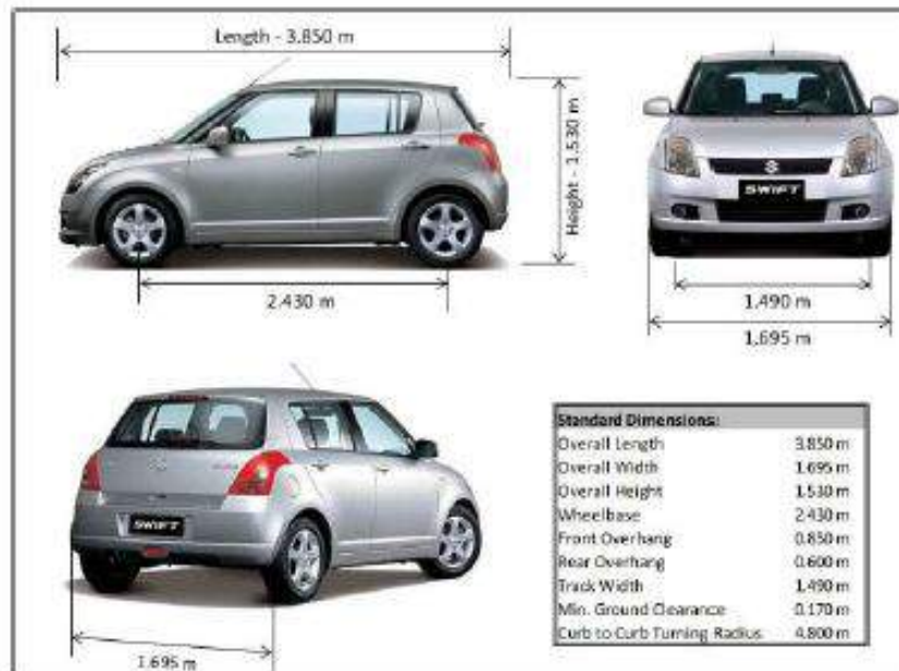
Figure 6-3 : Design Vehicle (Small Hatchback) – Maruti Suzuki Swift Dimensions
