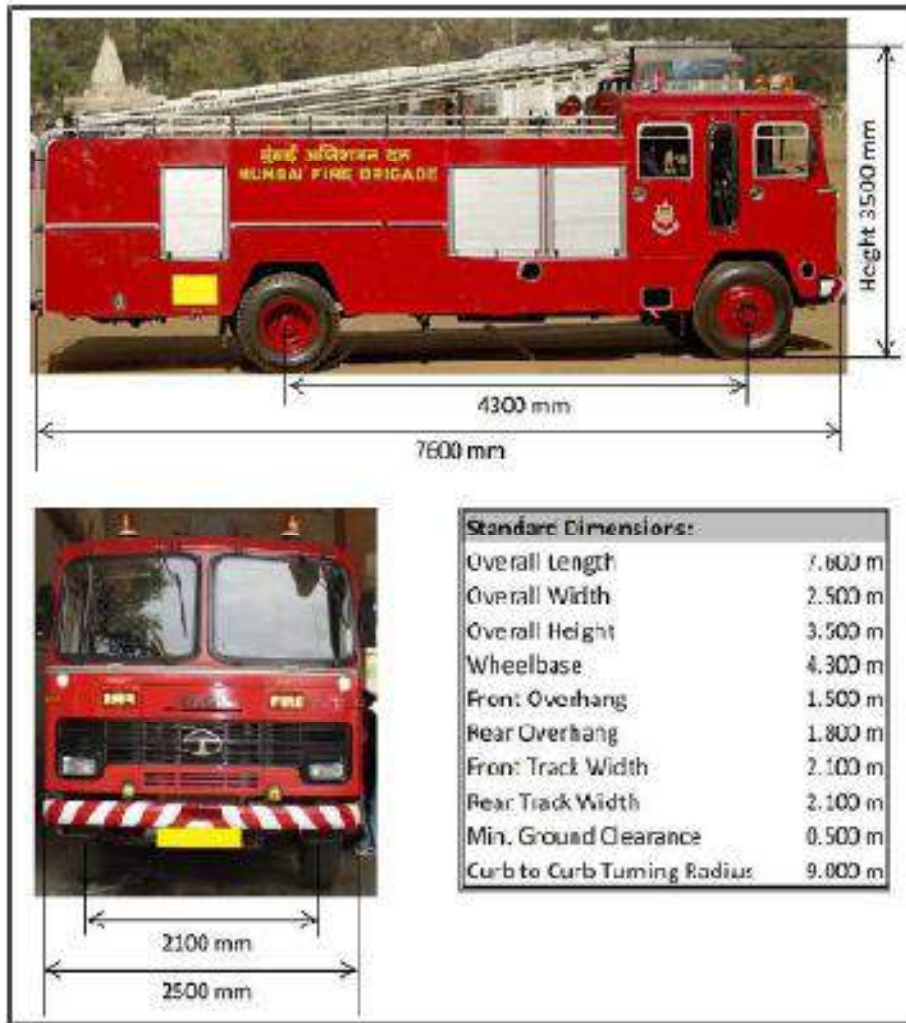
Figure 6-4 : Fire Tender Dimensions
